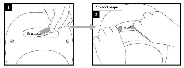
Place and keep one of the magnets on the swimmer symbol until the loud beep is heard, and until the red indicator light flashes quickly, **then** move the 2<sup>nd</sup> magnet over the red Stop symbol. The red indicator light remains on during the confirmation sound signal (15 short beeps).
