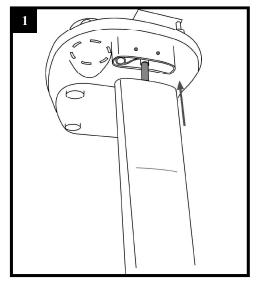
Carefully insert the rigid tube to a sufficient depth (about 3 cm).
