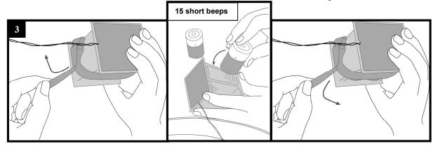
Insert the batteries, making sure the polarity is respected. Validation sound signal (15 short, high-pitched beeps). Your device is in "Off" mode.
