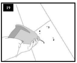
Drill the 4 holes with a  $\emptyset$  8mm bit.
