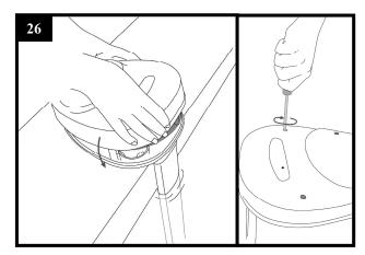
Replace the cover, and tighten the 4 screws again.
