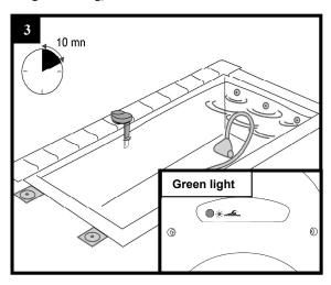
Filtering and robot cleaner working for 10 minutes, your immersion detector is monitoring (green indicator light flashing).
