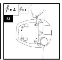
Tighten the 4 screws with their washers (provided with the attachment kit).
