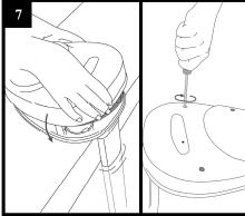
Replace the cover, and tighten the 4 screws again.
