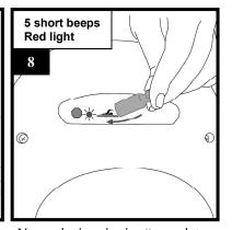
Your device is in "complete stop" mode, you must activate it and check that it is operating properly by carrying out the validation tests again (see item 3.7).
