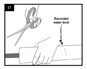
Cut the black tube flush with the rigid tube, using shears or heavy-duty scissors.
