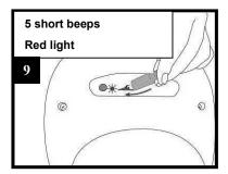
Your device is in "complete stop" mode, and must be activated for the installation tests.
