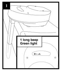
Your immersion detector is in monitoring mode (green indicator light flashing)
