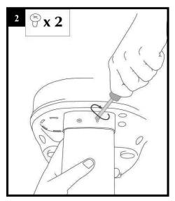
Screw the 2 self-drilling screws (provided with the attachment kit)
