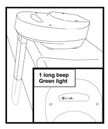
Your immersion detector is in monitoring mode (green indicator light flashing) Your immersion detector continuously checks the pool disturbance conditions.
