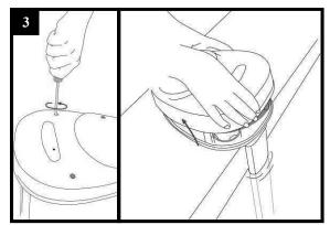
Unscrew the 4 screws and remove the cover.
