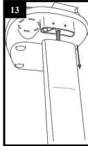
Carefully remove the rigid tube. DO NOT REMOVE THE BLACK TUBE
