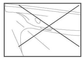
Joint excessively compressed.
