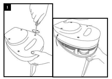
Unscrew the 4 screws and remove the cover.
