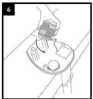
Replace the battery block on the Velcro strip.
