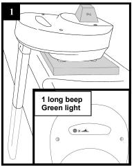
Your immersion detector is in monitoring mode (green indicator light flashing)
