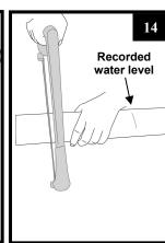
Firmly hold the rigid tube while cutting with the hacksaw.
