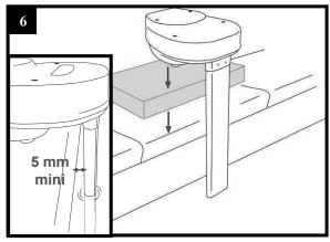
If your immersion depth is greater than 25 cm, use a booster (book, flat stone, brick, wooden board, etc.) which must not destabilize the central unit.
