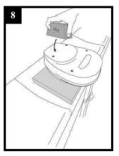
Carefully place a 2 to 3 kg weight on the device to hold it in place.
