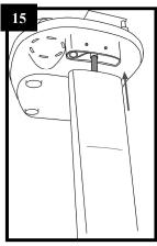
Carefully replace the tube by pushing it in deep enough (about 3 cm): Align the 2 holes already drilled.
