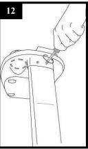
Unscrew the 2 screws holding the rigid tube.
