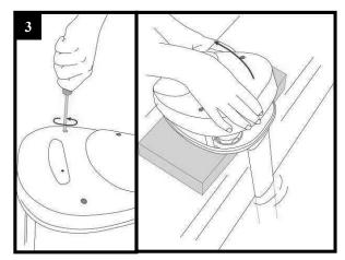
Unscrew the 4 screws and remove the cover.
