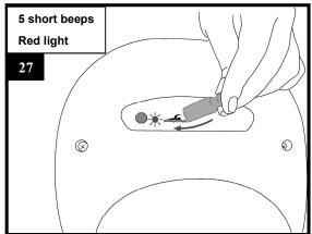
Your device is in "complete stop" mode, and must be activated for the validation tests.
