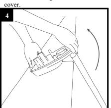
Remove the device and the booster from the coping.
