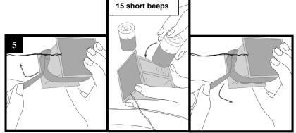
Replace the 4 batteries, making sure the polarity is respected. Validation sound signal (15 short, high-pitched beeps). Your device is in "Off" mode.
