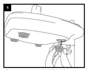
Remove the 4 pieces of stabilizing foam.
