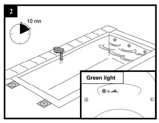
Filtering working for 10 minutes, your immersion detector is monitoring (green indicator light flashing).
