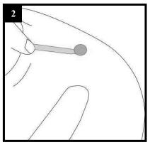
Carefully remove the 4 caps using a flat screwdriver.
