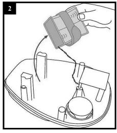
Remove the battery block fastened by a Velcro strip.
