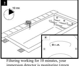
immersion detector is monitoring (green indicator light flashing).
