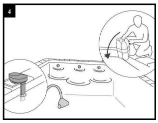
With the filtering system and robot cleaner working, drop the 6 kg weight from the top of the coping, from the point furthest away from your immersion detector.
