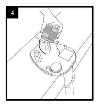
Remove the battery block fastened by a Velcro strip.
