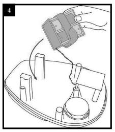
Replace the battery block on the Velcro strip.
