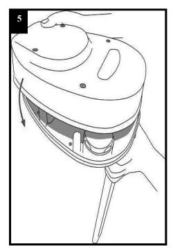
Replace cover without tightening the screws.
