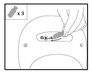
To manually start and stop the tests mode, place and keep the magnet on the swimmer symbol **until the loud beep is heard** and until the red indicator light flashes quickly.
