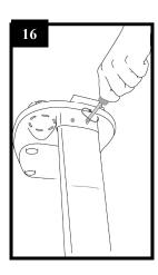
Tighten the 2 screws holding the tube.
