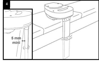
The rigid tube must be at least 5 mm from the edge of the coping.
