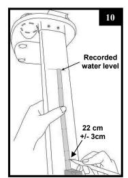
Using the measuring tape, measure the immersion depth from the water level. This must be between 19 cm and 25 cm (ideally 22 cm).
