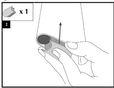
Place the wedge plug (included in the attachment kit) at the end of the tube.
