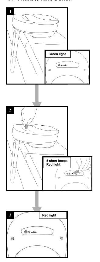
While the immersion detector is monitoring (green indicator light), move the magnet over the swimmer symbol in the activation area of your device:
