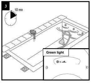
Filtering and robot cleaner working for 10 minutes, your immersion detector is monitoring (green indicator light flashing) and must not set off the alarm.
